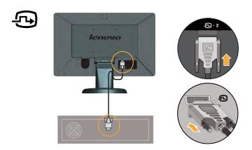
4. Insert the power cord into the monitor, then plug the monitor power cord and the computer cord into grounded electrical outlets.
